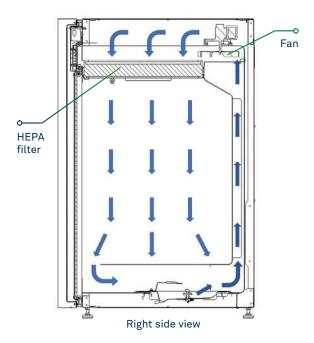
Air flows down to the chamber bottom, under the false floor, passing over the humidity source. The fan pulls air tap behind the rear baffle to the top of the unit, where it passes through a full-face HEPA filter, delivering clean, better-than-ISO Class 4 (Class 10) air.
