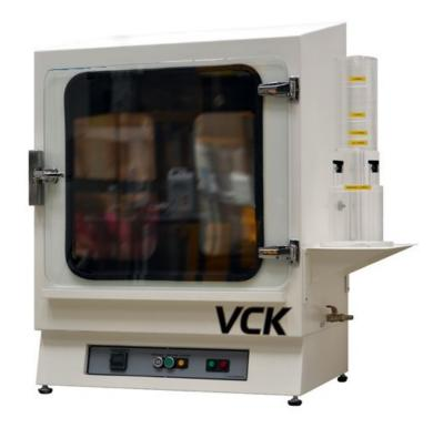
The Kesternick Corrosion Test has been designed to simulate industrial or urban atmospheres by means of the creation of an artificial atmosphere, by adding Sulphurous Anhydrid to the air, with or without Carbon Dioxide.
