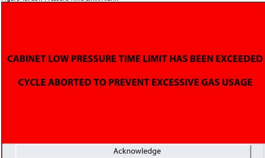
Figure 43: Low Pressure Time Limit Alarm
