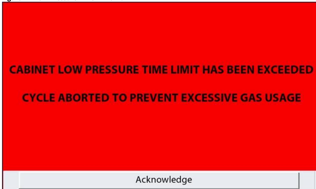
Figure 41: Low Pressure Time Limit Alarm
