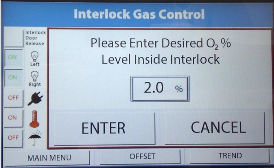
Figure 61: Interlock O 2 desired level
