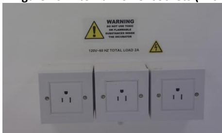
Figure 16: Internal Power sockets (120V) Internal Power sockets (230V)
