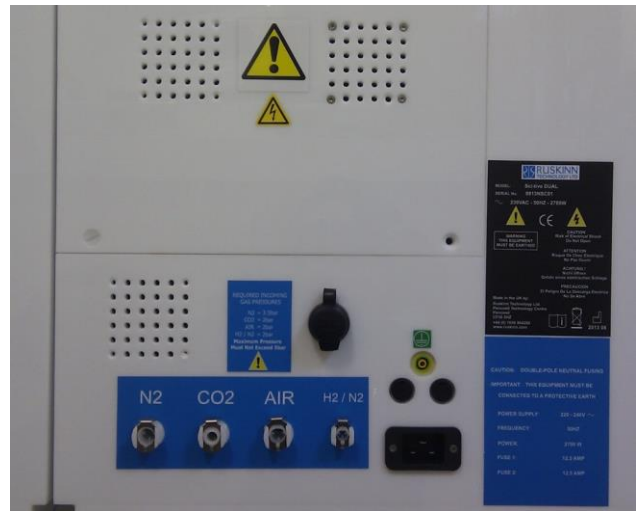
Figure 4: Gas and electrical connections (230V)
