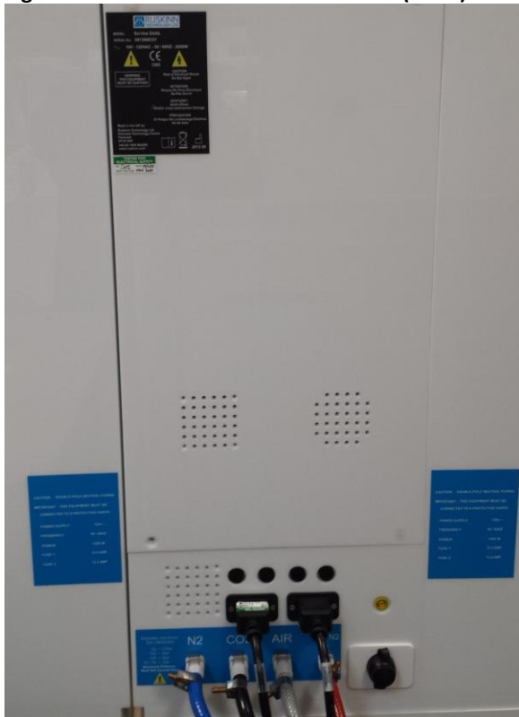
Figure 3: Gas and electrical connections (120V)
