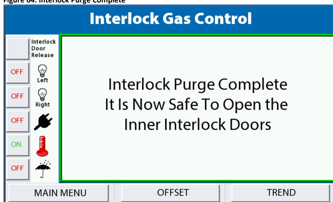
Figure 64: Interlock Purge Complete
