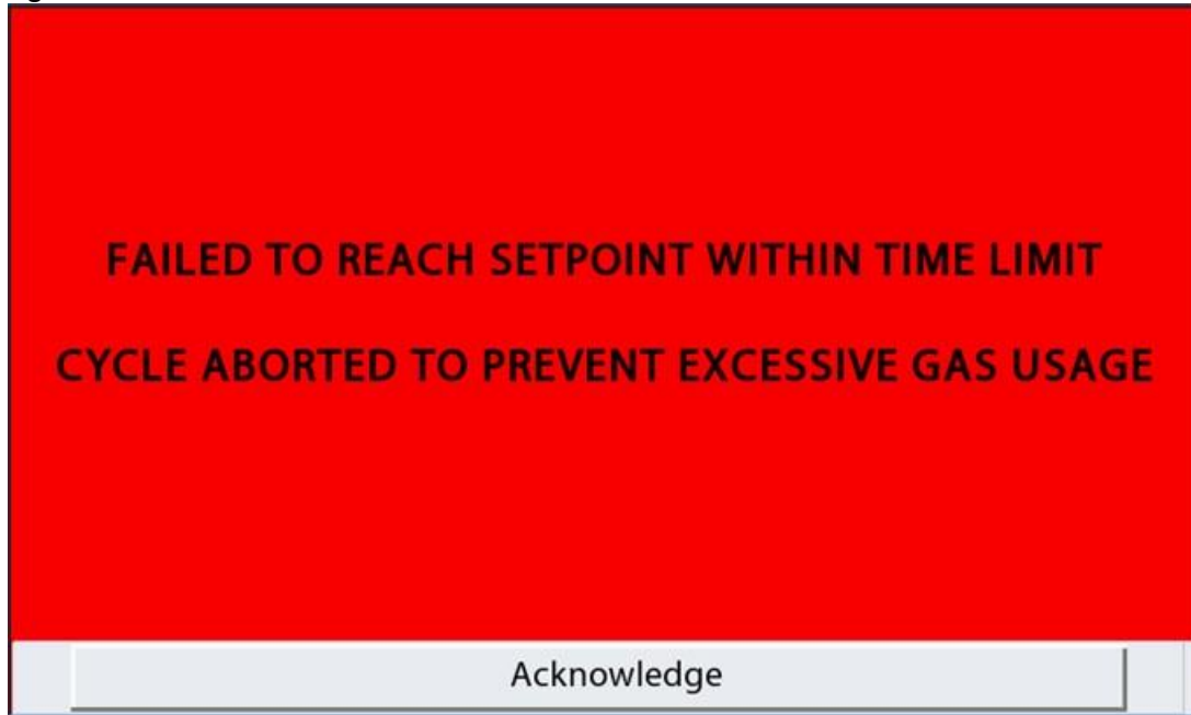
Figure 40: Failure to reach Set Point Alarm
