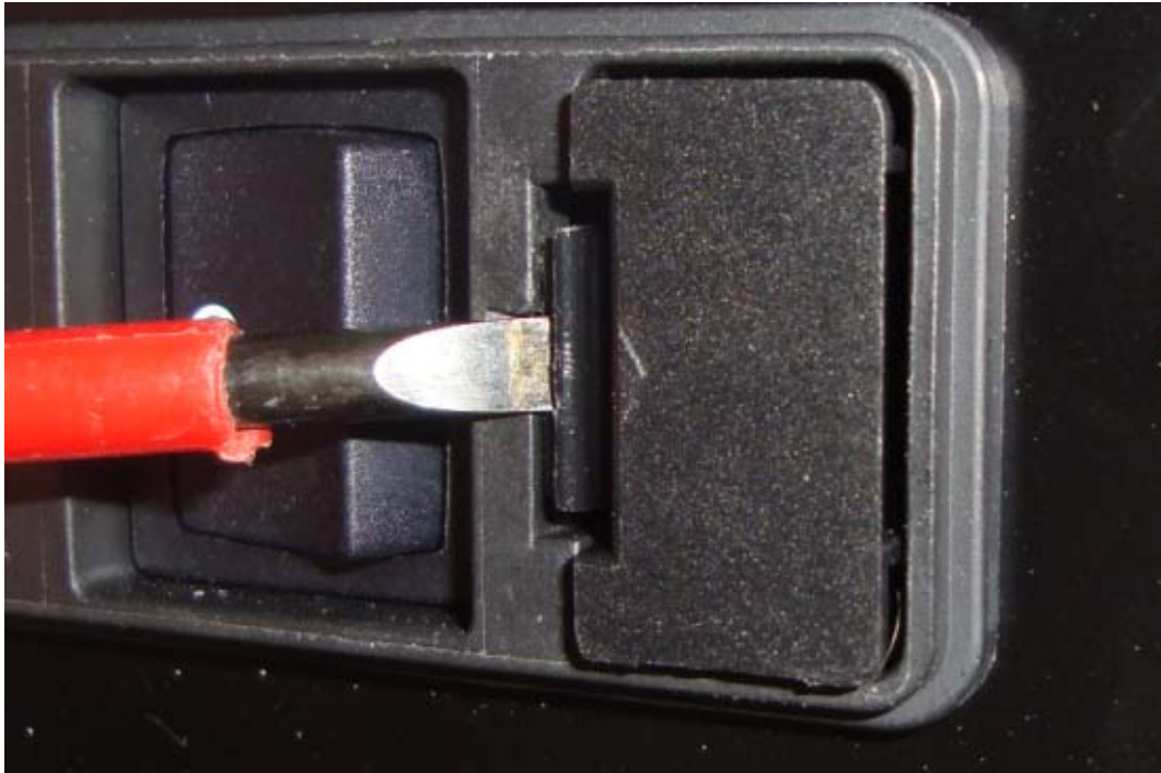
Figure 28: Mains fuse holder removal
