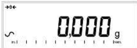
A stable sign **~** is shown when the analyzer is in stable condition. It will turn off if the analyzer is not stable. Exact zero is shown when the "**→0←**" symbol is on to the left of the display area.
