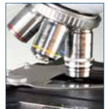
S100x objective with built-in iris diaphragm
