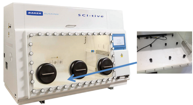
Figure 1. SCI-tive (left) with inset showing ferrules that support the internal floor tray (right).
