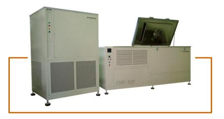
\_This equipment is compounded by two modules: freezer cabinet (where place the samples to be tested). Thermostatic bath (where acclimate the water to do the freeze-thaw cycles with water). Dycometal equips the cabinets with a potent microprocessor, which has a high number of programs for carrying the tests for the building materials. Bibliography<sup>1</sup>
