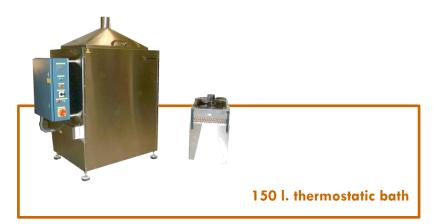
1\_lt's usual to equip these equipments with a condenser in order to maintain the temperature water between  $18-25^{\circ}$ C. Also, in equipments which can regulate the temperature till  $90/100^{\circ}$ C, the cover is usually designed with an angle and one chimney to vent the vapors. To obtain a good homogeneity of the water, it's added a heating pump which recirculates the water in a constant form. The heaters will be in the base of the bath, and they are protected by a holed sheet.
