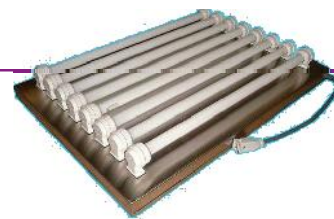
Lighting system for photostability tests
